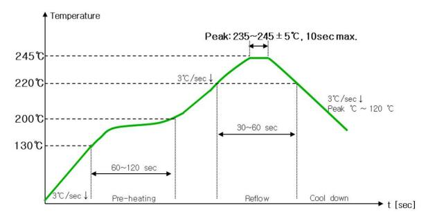
Figure 7: DWM1001 Module Solder Profile
