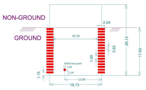
Figure 6: DWM1001 Module Land Pattern (units: mm)
