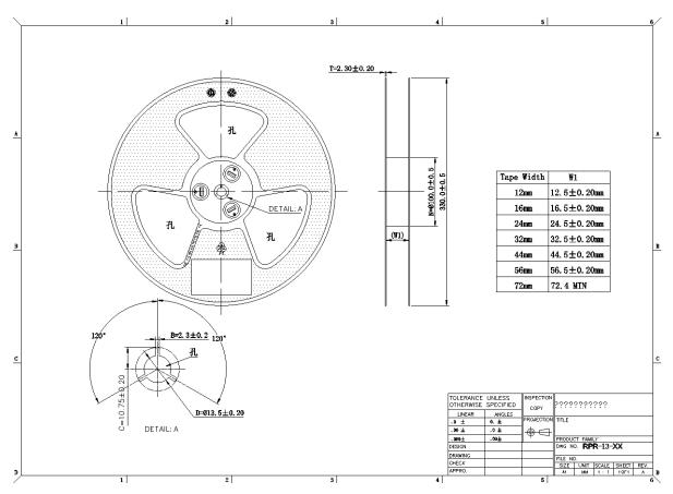
Figure 8: DWM1001 Tape and Reel Dimensions
