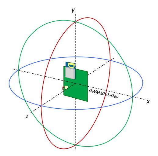
Figure 3. Antenna Radiation Pattern Planes
