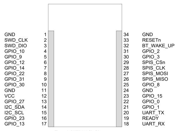
Figure 1: DWM1001 Pin Diagram
