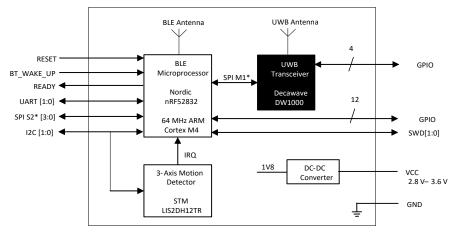
\*SPI M1 is nRF52 SPI master 1, SPI S2 is SPI slave 2
