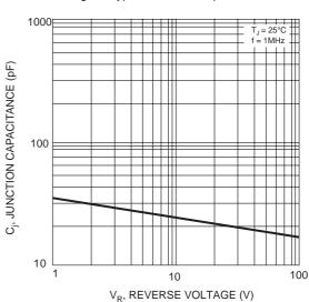
Fig. 4 Typical Junction Capacitance
