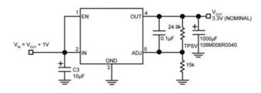
Figure 2. IFX1963 Load Transient Response Test Circuit
