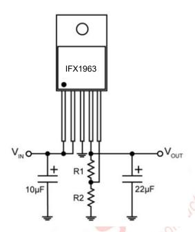
Figure 4. Adjustable Regulator with Resistors
