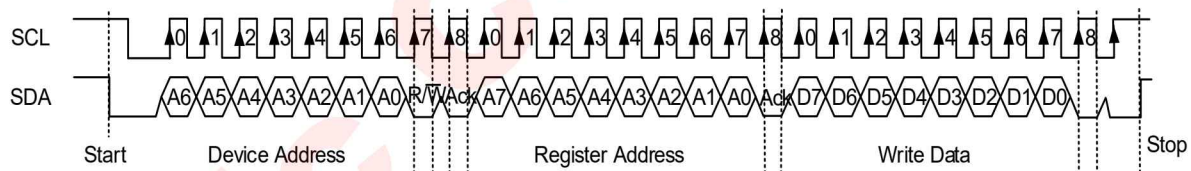
Figure 6 I 2 C Write Byte Cycle
