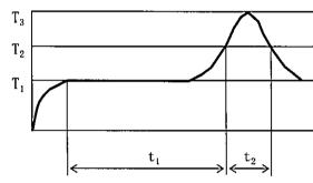
$T_1=150$  to  $180^{\circ}$ C  $T_2=230^{\circ}$ C  $T_3=250^{\circ}$ C or less  $t_1=60$  to 120s or less  $t_2=30s$  or less
