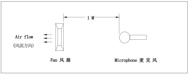
(在背景噪音不超过 18dB (A) 的无响室内,将待测风扇通入额定的工作电压,悬掉入空中,将麦克风放于风扇同一平面且离待测风扇进风口一米处进行测试其 B&K 值) Noise is measured rated voItage in free air in anechoic chamber with B&K sound IeveI meter with microphone at a distance of one meter from the fan intake. The background noise is 18Db(A) max。
