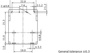
$Note: Terminal\ dimensions\ are\ values\ without\ pre-soldering\ thickness.$
