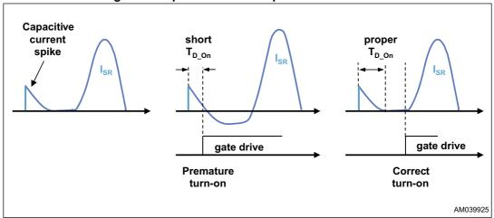
Figure 6. Capacitive current spike effect at turn-on
