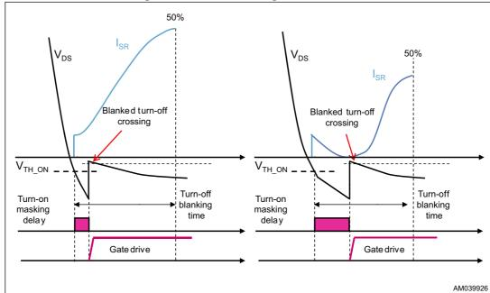
Figure 7. Full load and light load turn-on
