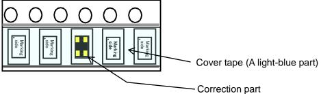
2. A cover tape is cut along the part of a red line. (3 sides)
