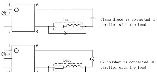
2) Clamp diode or CR Snubber can limit spike voltages from the load. However, the inductance increases by long wiring and it may cause spike voltages. Please keep the wire as short as possible to minimize inductance.
