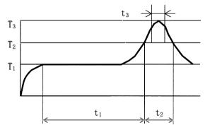
$T_1$ =150 °C to 180 °C  $T_2$ =230 °C  $T_3$ =240 °C to 250 °C  $t_1$ =60 s to 120 s  $t_2$ =Within 30 s  $t_3$ =Within 10 s
