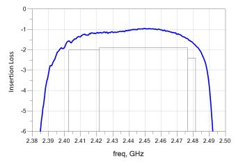
Figure.1 Passband Insertion Loss
