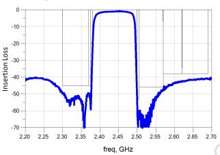
Figure.3 Narrowband Insertion Loss
