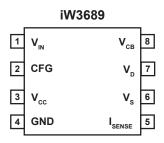
Figure 4.1: 8-Lead SOIC-8 Package
