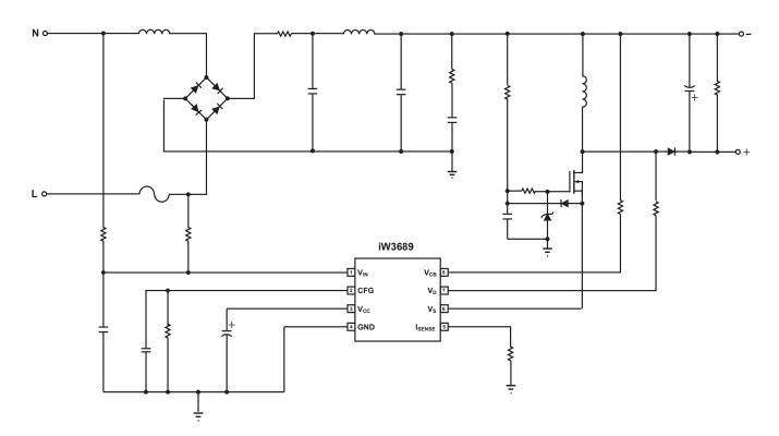
Figure 3.1: iW3689 Typical Application Circuit
