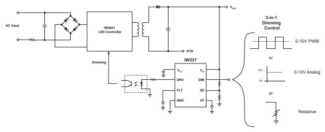
Figure 3.1: iW337 Typical Application Circuit
