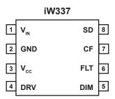
Figure 4.1: 8-Lead SOIC Package
