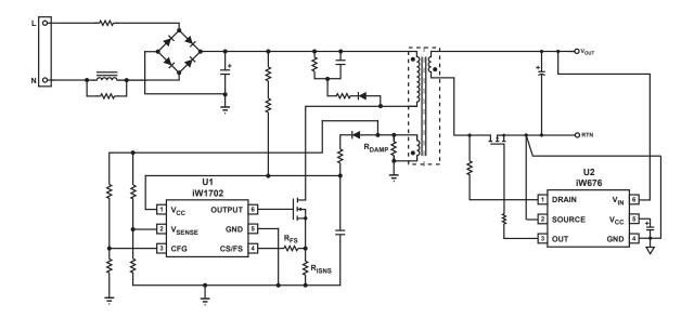
Figure 3.4 : iW1702 Typical Application Circuit with Supplement Output Over-Voltage Protection and iW676-32C Secondary Synchronous Rectifier Controller with Active Voltage Positioning.
