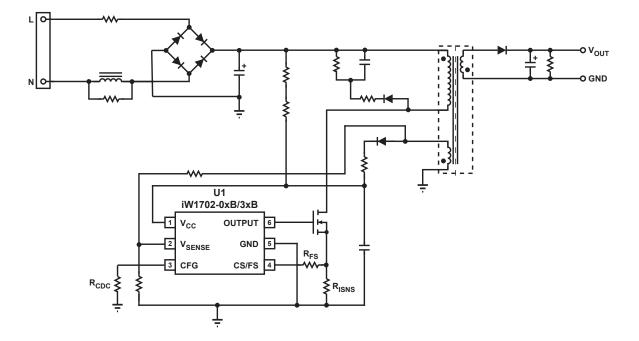
Figure 3.1 : iW1702 Typical Application Circuit (Achieving < 75mW No-Load Power Consumption in 12V, 2A 24W Adapter Design).
