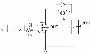
3) Switch Time Test Circuit
