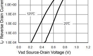
Figure 6 Source- Drain Diode Forward
