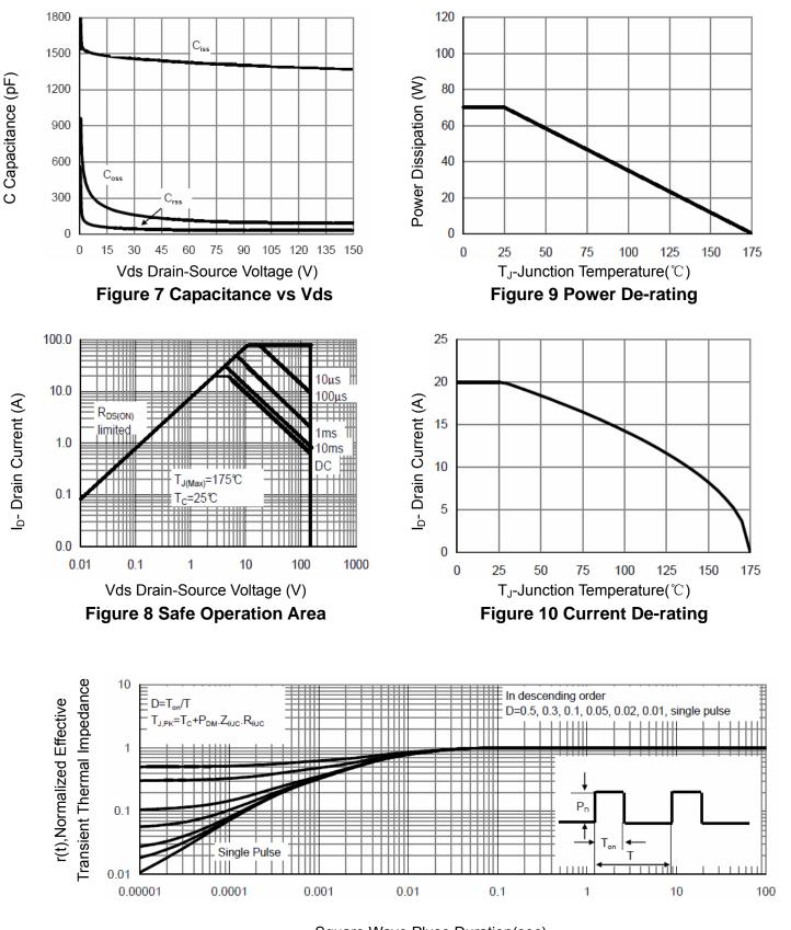
Square Wave Pluse Duration(sec) Figure 11 Normalized Maximum Transient Thermal Impedance
