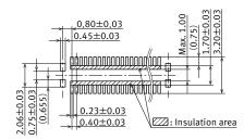
Recommended metal mask pattern Metal mask thickness: When 150 µm (Terminal opening ratio: 48%) (Metal-part opening ratio: 100%)
