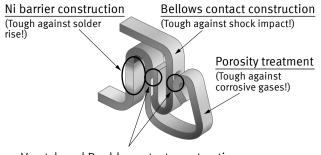
V notch and Double contact constructions (Tough against exposure to foreign particles and solder flux!)
