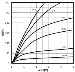
Figure 1. Type. Output Characteristics (Tj=25 ℃)
