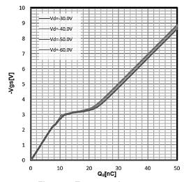
Figure 7. Typ. gate charge VGS =f(Q gate); ID =20A
