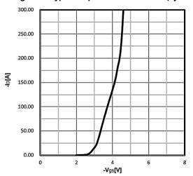
Figure 3. Type. transfer characteristics
