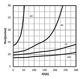
Figure 2. Type. drain-source on resistance
