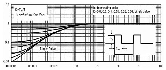
Figure 10. Max. transient thermal impedance ZthJC =f(tp)
