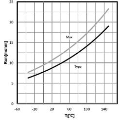
Figure 5. Drain-source on-state resistance RDS(on) =f(Tj); ID =80A; VGS =10V
