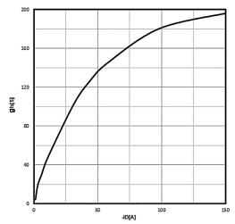
Figure 4. Type. forward transconductance
