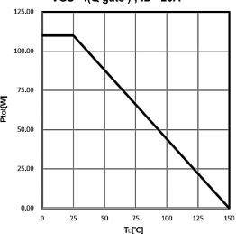
Figure 7. Power Dissipation
