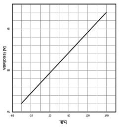
Figure 8. Drain Current Derating VBR(DSS) = f(T j ); I D = 250uA
