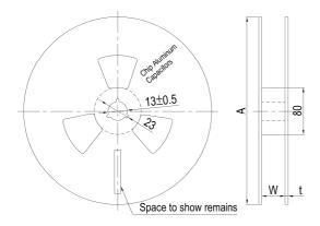
Fig. 2-2 Reel Polarity
