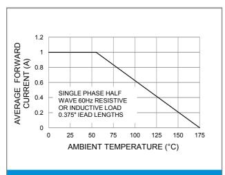
Fig.1 FORWARD CURRENT DERATING CURVE
