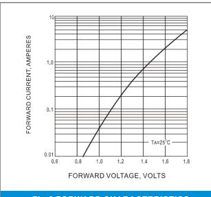
Fig.3 FORWARD CHARACTERISTICS
