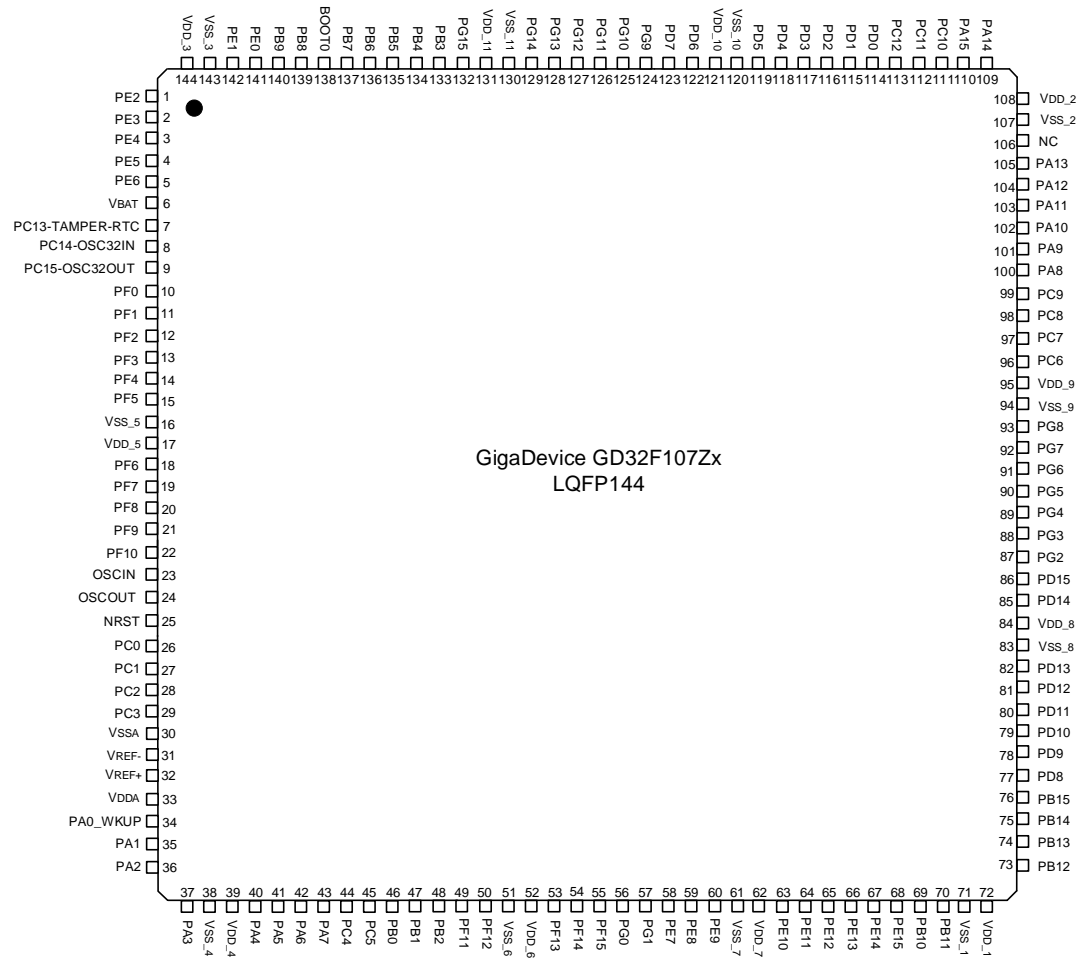
Figure 2-2. GD32F107Zx LQFP144 pinouts
