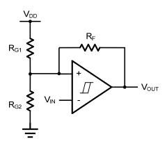
Figure 4. Inverting Comparator with Hysteresis
