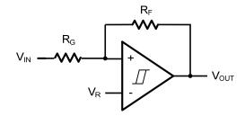
Figure 3. Non-Inverting Comparator with Hysteresis
