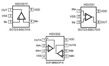
Figure 1. Pin Assignment Diagram
