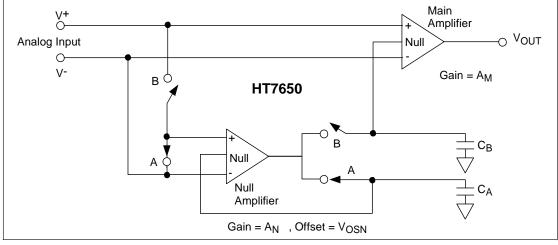
FIGURE 3-2: NULLING CAPACITOR CONNECTION
