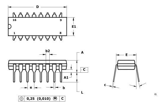
Note - Dimensions D, E1 do not include the fin value, which should not exceed 0.25 mm (0.010) per side.
