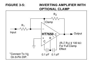
The output clamp circuit is shown in Figure 3-3, with typical inverting and non-inverting circuit connections shown in Figures 3-4 and 3-5. Output voltage versus clamp circuit current characteristics are shown in the typical operating curves. For the clamp to be fully effective, the impedance across the clamp output should be greater than  $100 k\Omega$ .
