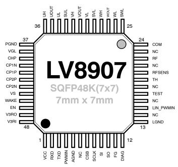
Figure 4. LV8907 Pinout
