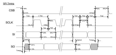
Figure 16. SPI Timing Chart
