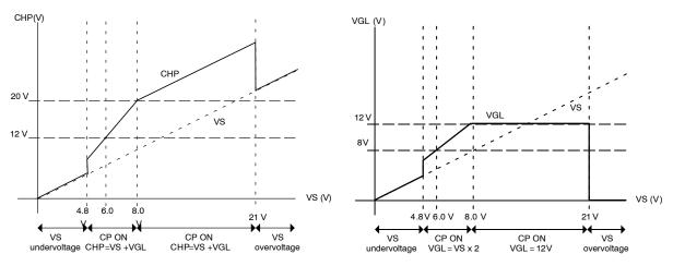
Figure 9. High-side and Low-side Gate Voltages
