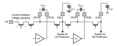
Figure 8. Charge Pump Circuit
