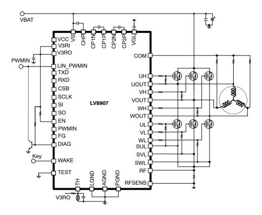
Figure 2. Example of Stand-alone Configuration
