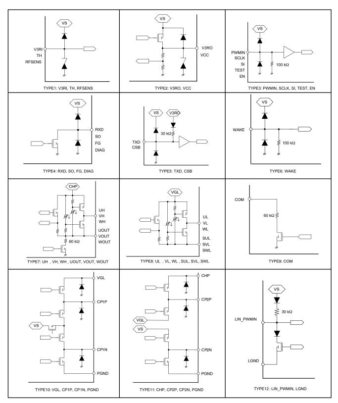
Figure 5. Pin Circuit
