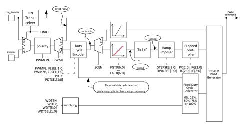
Figure 12. PWM Command Flow and Related Registers
