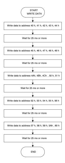
Figure 24. OTP Memory Write Operation
