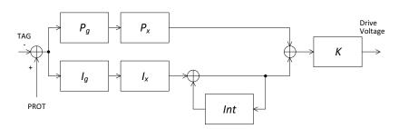
Figure 18. PI Speed Controller Block Diagram
