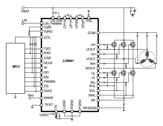
Figure 3. Example of LIN Based Control Configuration
