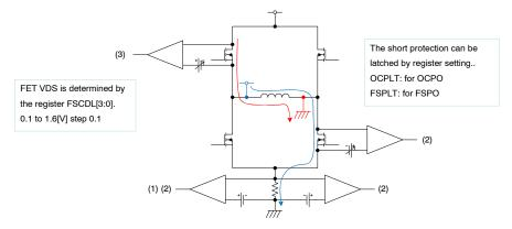
Figure 13. Current Limit vs. Overcurrent Shutoff
