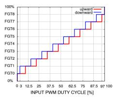
Figure 11. Target Speed Register Selection by Input PWM Duty Cycle
