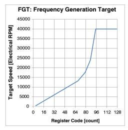
Figure 19. Speed Register Contents vs. Electrical RPM
