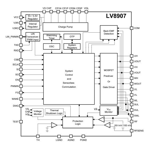
Figure 1. LV8907 Block Diagram
