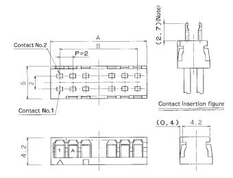
Note: The dip side may be deviated according to the cable thickness and the crimping contact bent up/down.
