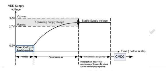
Host needs to keep power line level less than 0.5V and more than 1ms before power ramp up.
