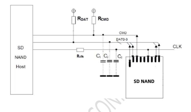
RDAT and RCMD (10K~100 k $\Omega$ ) are pull-up resistors protecting the CMD and the DAT lines against bus floating when SD NAND is in a high-impedance mode.
