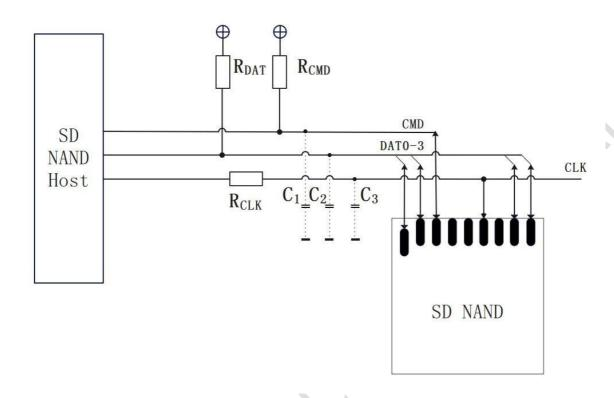
RDAT and RCMD (10K $\sim$ 100 k $\Omega$ ) are pull-up resistors protecting the CMD and the DAT lines against bus floating when Nano SD NAND is in a high-impedance mode.
