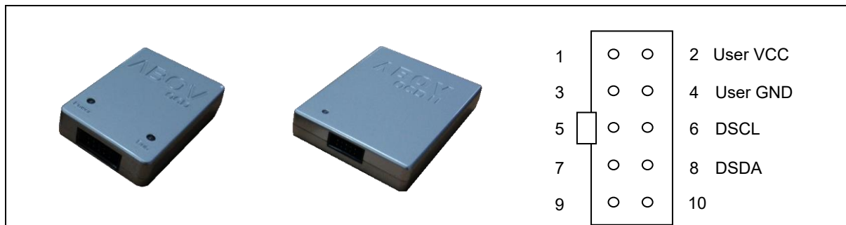
Figure 31. Debugger (OCD1/OCD2) and Pinouts
