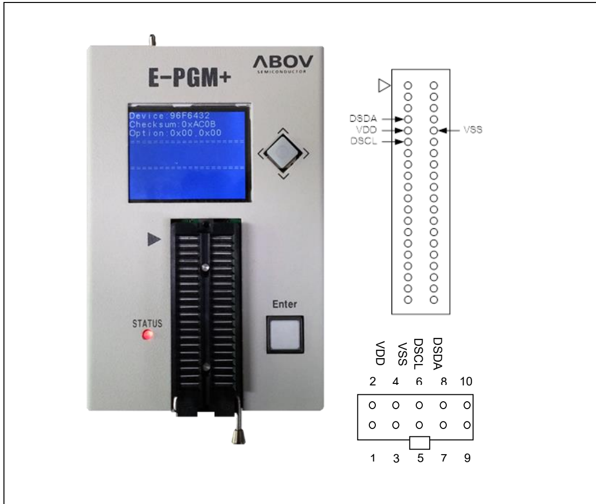
Figure 40. E-PGM+ (Single Writer) and Pinouts
