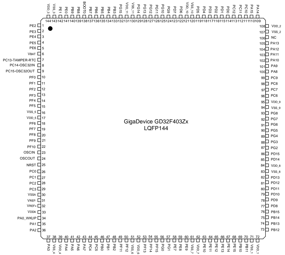
Figure 2-2. GD32F403Zx LQFP144 pinouts
