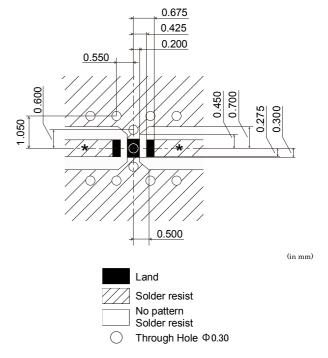
$<sup>^{\</sup>star}$  Line width to be designed to match 50 ohm characteristic impedance, Depending on PCB material and thickness.
