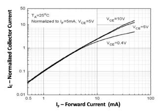
Fig 3 Normalized Collector Current vs Forward Current
