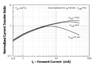
Fig 4 Normalized Current Transfer Ratio vs Forward Current
