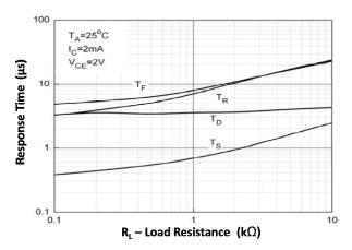
Fig 10 Response Time vs Load Resistance
