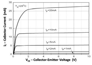
Fig 1 Collector Current vs Collector-Emitter Voltage
