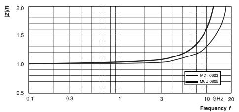
Relative impedance for 49.9  $\Omega$  chip resistor
