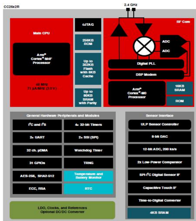
Figure 1-1. CC2642R Block Diagram
