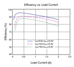
Figure 2. Efficiency Figure
