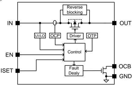
Figure 2. Block Diagram
