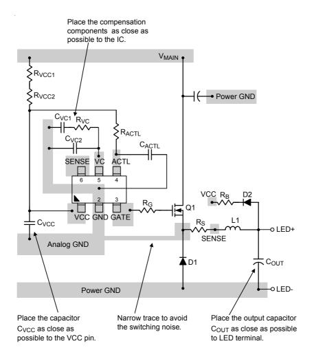
Figure 2. PCB Layout Guide
