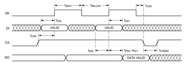
Figure 2. Synchronous Data Timing
