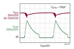
Figure 1. Charge Current Waveform for V<sub>SCAP</sub> <1V
