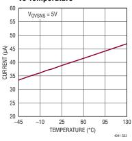
Supercapacitor Balancer Source/Sink Current
