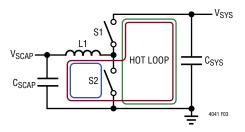
Figure 3. Hot-Loop Illustration for the LTC4041 Switching Converter
