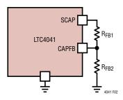
Figure 2. Programming the Charge Voltage
