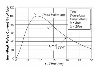
Fig2. Pulse Waveform
