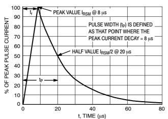
Figure 4. 8 X 20 µs Pulse Waveform
