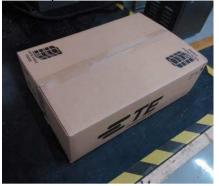
After Test: Carton corner was out of shape, but no broken. Inner packaging was OK. Parts were OK.
