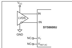
FIGURE 7-5: LVDS Interface (DC-Coupled).
