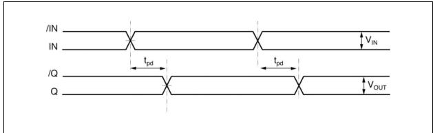
FIGURE 3-1: Propagation Delay.
