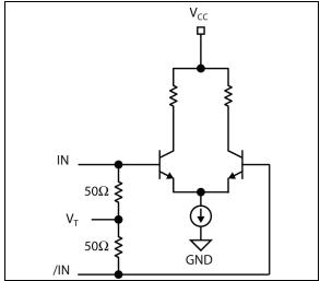
FIGURE 6-1: Simplified Differential Input Buffer.
