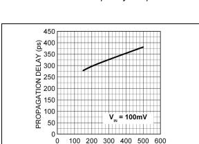
FIGURE 4-2: Propagation Delay vs. Input Rise/Fall Time.
