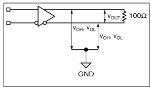
FIGURE 6-3: LVDS Differential Measurement.
