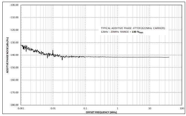
FIGURE 5-1: Additive Noise Plot.
