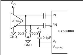
FIGURE 7-4: LVPECL Interface (AC-Coupled).
