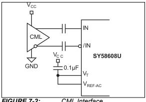
FIGURE 7-2: CML Interface (AC-Coupled).
