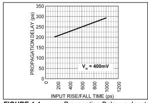
**FIGURE 4-4:** Propagation Delay vs. Input Rise/Fall Time.
