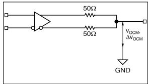
FIGURE 6-5: LVDS Common Mode Measurement.
