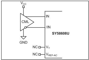
FIGURE 7-1: CML Interface (DC-Coupled).
