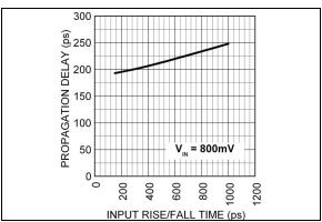
FIGURE 4-5: Propagation Delay vs. Input Rise/Fall Time.
