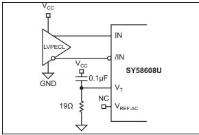
FIGURE 7-3: LVPECL Interface (DC-Coupled).
