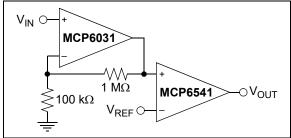
FIGURE 4-8: Precision, Noninverting Comparator.
