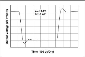
**FIGURE 2-29:** Small-Signal Inverting Pulse Response.
