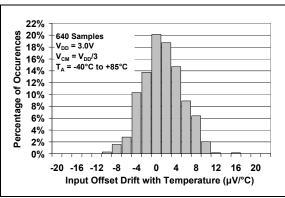
**FIGURE 2-2:** Input Offset Voltage Drift with  $V_{DD} = 3.0V$  and  $T_A \le +85^{\circ}C$ .
