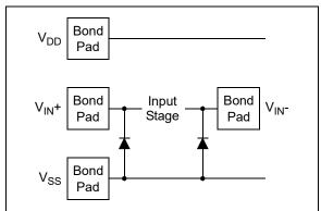
FIGURE 4-1: Simplified Analog Input ESD Structures.
