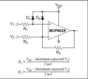
FIGURE 4-2: Protecting the Analog Inputs.
