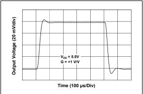
**FIGURE 2-28:** Small-Signal Noninverting Pulse Response.
