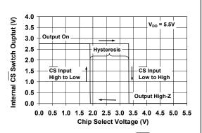
**FIGURE 2-34:** Chip Select ( $\overline{CS}$ ) Hysteresis (MCP6033 only) with  $V_{DD} = 5.5V$ .
