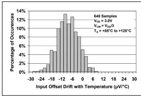
**FIGURE 2-3:** Input Offset Voltage Drift with  $V_{DD} = 3.0V$  and  $T_A \ge +85^{\circ}C$ .
