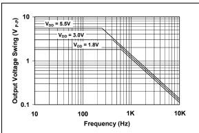
FIGURE 2-24: Output Voltage Swing vs. Frequency.
