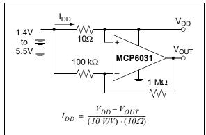
FIGURE 4-7: High-Side Battery Current Sensor.
