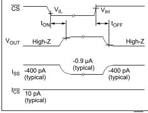
**FIGURE 1-1:** Timing Diagram for the  $\overline{\text{CS}}$  Pin on the MCP6033.
