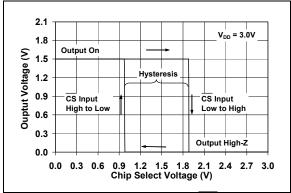
**FIGURE 2-35:** Chip Select (CS) Hysteresis (MCP6033 only) with  $V_{DD} = 3.0V$ .
