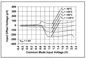
**FIGURE 2-5:** Input Offset Voltage vs. Common-mode Input Voltage with  $V_{DD} = 1.8V$ .
