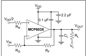
FIGURE 1-3: AC and DC Test Circuit for Most Inverting Gain Conditions.
