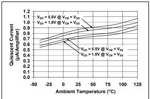
**FIGURE 2-13:** Quiescent Current vs Ambient Temperature.
