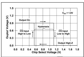
**FIGURE 2-36:** Chip Select (CS) Hysteresis (MCP6033 only) with  $V_{DD} = 1.8V$ .
