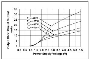
**FIGURE 2-23:** Ouput Short-Circuit Current vs. Power Supply Voltage.
