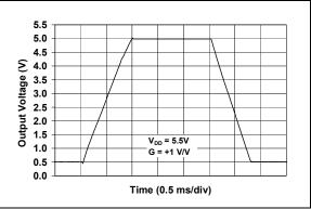
**FIGURE 2-30:** Large-Signal Noninverting Pulse Response.
