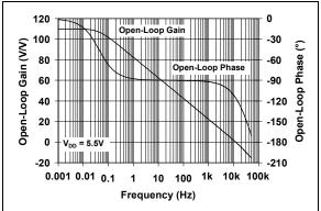
**FIGURE 2-16:** Open-Loop Gain, Phase vs. Frequency.
