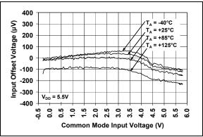
**FIGURE 2-4:** Input Offset Voltage vs. Common-mode Input Voltage with  $V_{DD} = 5.5V$ .
