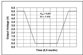
**FIGURE 2-31:** Large-Signal Inverting Pulse Response.
