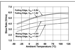
FIGURE 2-27: Slew Rate vs. Ambient Temperature.
