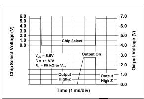
FIGURE 2-33: Chip Select (CS) to Amplifier Output Response Time (MCP6033 only).
