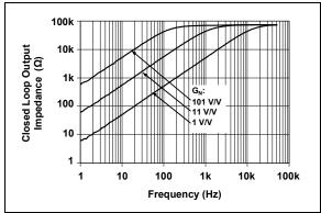
FIGURE 2-37: Closed-Loop Output Impedance vs. Frequency.
