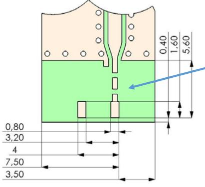
All metallization should be removed from all PWB layers.
