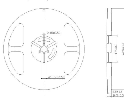
Dimensions of Tape (Unit: mm)
