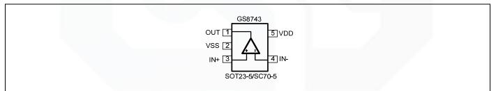
Figure 1. Pin Assignment Diagram
