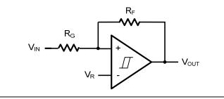
Figure 3. Non-Inverting Comparator with Hysteresis
