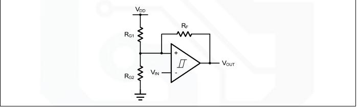
Figure 4. Inverting Comparator with Hysteresis
