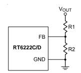
Figure 5. Output Voltage Setting
