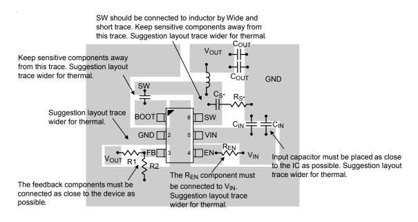
Figure 8. PCB Layout Guide
