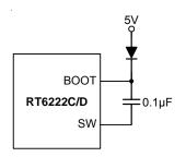
Figure 6. External Bootstrap Diode
