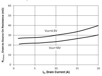
Fig. 4 On-Resistance vs. Gate to Source
