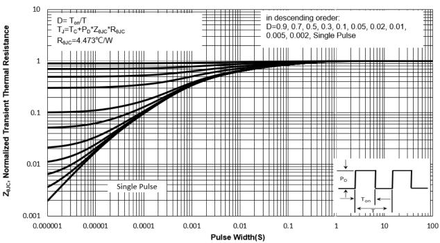
Fig.13 Normalized Maximum Transient Thermal Impedance(zeuc)
