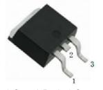
1.Gate 2.Drain 3.Source TO-252 Plastic Package
