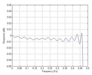
Figure 38: DAC Filter Ripple
