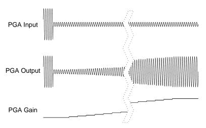
Figure 9: ALC Operation Without Noise Gate
