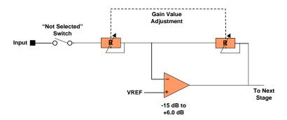
Figure 5: Variable Gain Stage Simplified Schematic
