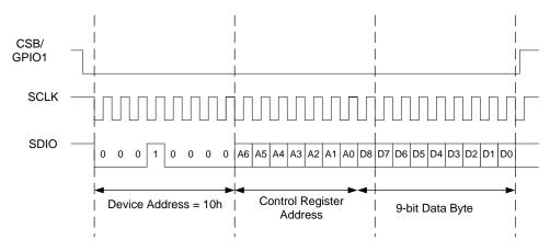
Figure 22: Register Write operation using a 24-bit SPI Interface
