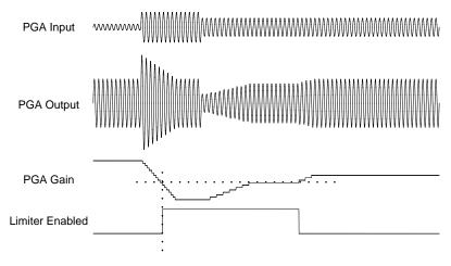
Figure 12: ALC Limiter Mode Operation
