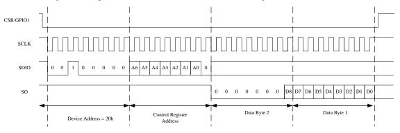
Figure 23: Register Read operation through a 32-bit SPI Interface
