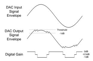
Figure 13: DAC Digital Limiter Control
