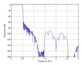
Figure 39: ADC Filter Frequency Response
