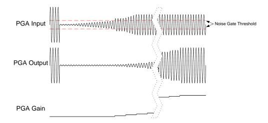
Figure 10: Noise Gate Operation
