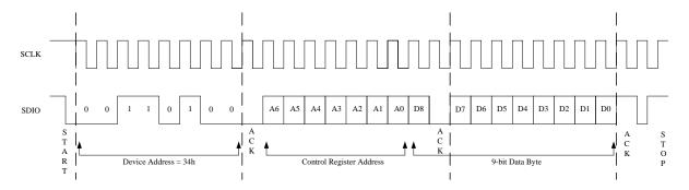
Figure 19: Byte Write Sequence
