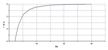
Figure 41: ADC Highpass Filter Response, Audio Mode
