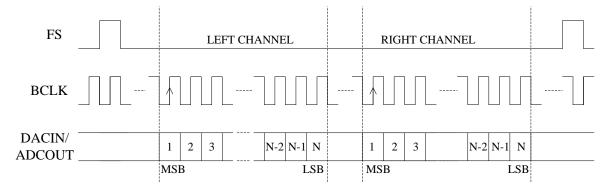
Figure 29: PCM Time Slot Audio Interface
