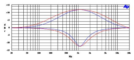
Figure 49: EQ Band 3, EQ3BW = 0 versus EQ3BW = 1
