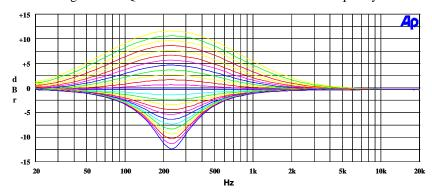
Figure 46: EQ Band 2 Peak Filter Gains for Lowest Cut-Off Frequency with EQ2BW = 0
