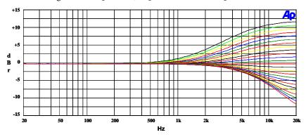
Figure 52: EQ Band 5 Gains for Lowest Cut-Off Frequency
