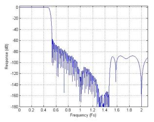
Figure 37: DAC Filter Frequency Response
