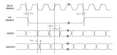
Figure 34: Digital Audio Interface Master Mode Timing
