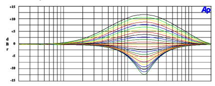
Figure 50: EQ Band 4 Peak Filter Gains for Lowest Cut-Off Frequencies with EQ4BW = 0
