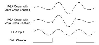
Figure 2: Zero Crossing Gain Update Operation
