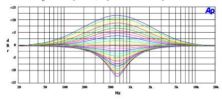
Figure 48: EQ Band 3 Peak Filter Gains for Lowest Cut-Off Frequency with EQ3BW = 0
