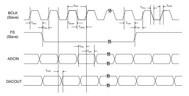
Figure 33: Digital Audio Interface Slave Mode Timing
