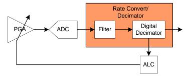
Figure 6: ALC Block Diagram
