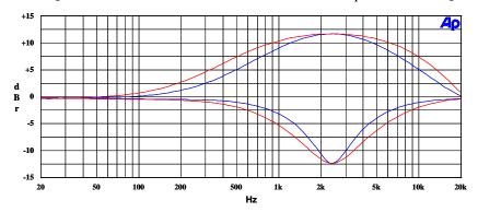
Figure 51: EQ Band 4, EQ4BW = 0 versus EQ4BW =1
