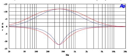
Figure 47: EQ Band 2, EQ2BW = 0 versus EQ2BW = 1
