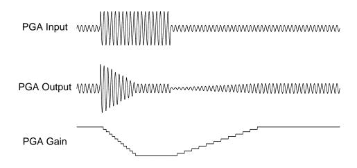
Figure 7: ALC Normal Mode Operation
