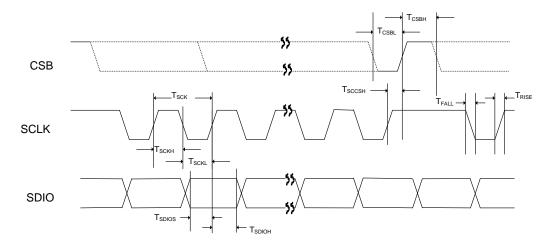
Figure 30: 3-wire ControlMode Timing
