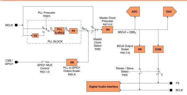
Figure 14: PLL and Clock Select Circuit
