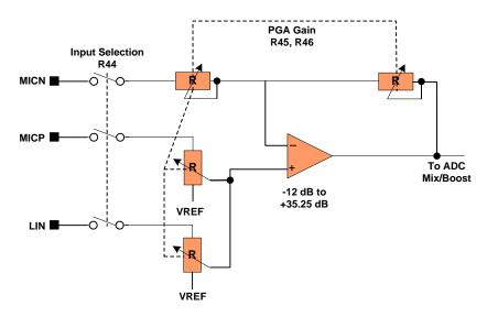
Figure 3: PGA Input Structure Simplified Schematic
