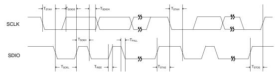
Figure 32: Two-wire Control Mode Timing
