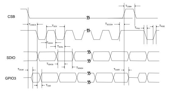
Figure 31: 4-wire ControlMode Timing
