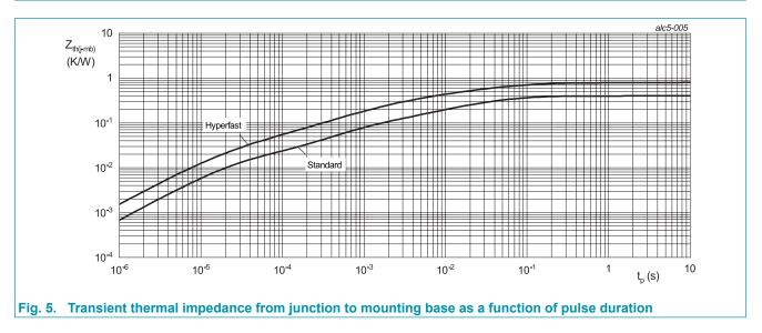
Hyperfast power diode with Standard recovery diode
