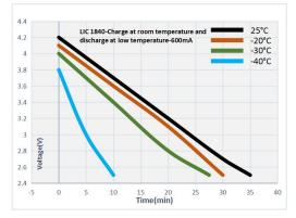
• Low internal resistance discharge characteristics-600mA
